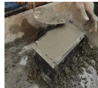
Fig 6 : Casting of brick
